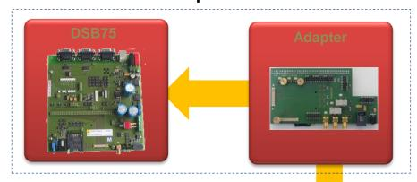
Combine DSB75 and Adapter for broadest testing scope including industry standard audio connectors, serial ports, USB and full-access to module pins
